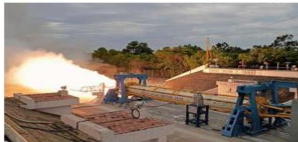
The ground test of the SOLVE solid motor being conducted at the Satish Dhawan Space Centre in Sriharikota. SPECIAL ARRANGEMENT
